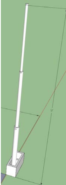
Figure 5.2.B: Webcam support structure.
