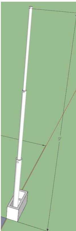
Figure 4.4.5.A: Google SketchUp model of the webcam support structure. Webcam will be mounted to the top of the pole, facing the lawn to be traversed.
