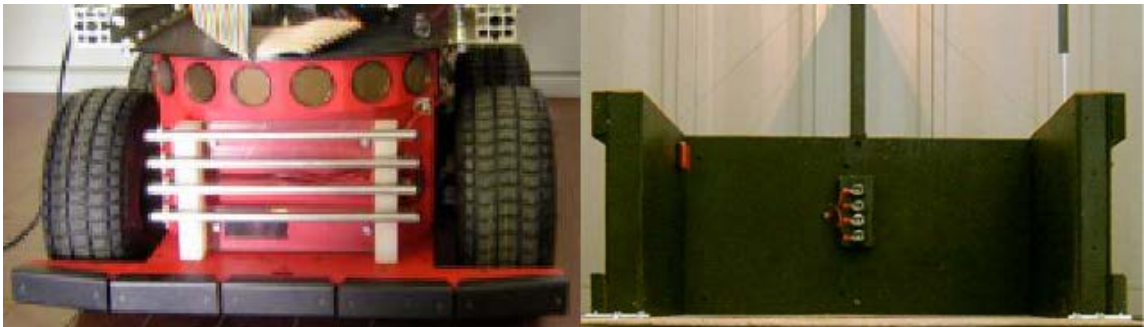
Figure 4.7.1.D - Charging contacts for robot and docking station. Reprinted with permission from Cassinis et al.
