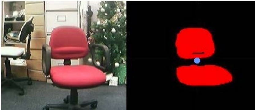
Figure 4.4.5.C: Left: input image. Right: output from blob detection algorithm. Reprinted with permission from John Palmisano ( www.societyofrobots.com ).
