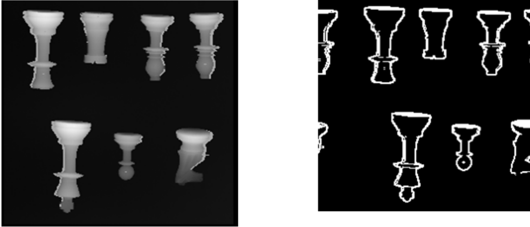
Figure 4.3.3.5.A: Low thresholding edge detection
