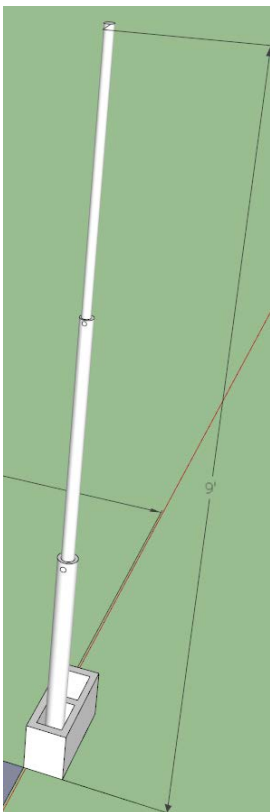
Figure 4.4.5.A: Google SketchUp model of the webcam support structure. Webcam was mounted to the top of the pole, facing the lawn to be traversed.
