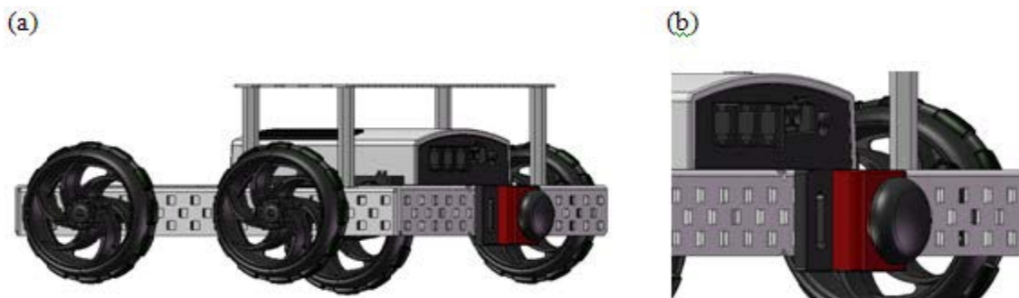
Figure 5.3.A - Design sample showing bumper sensor. Reprinted with permission from Vex Robotics.
