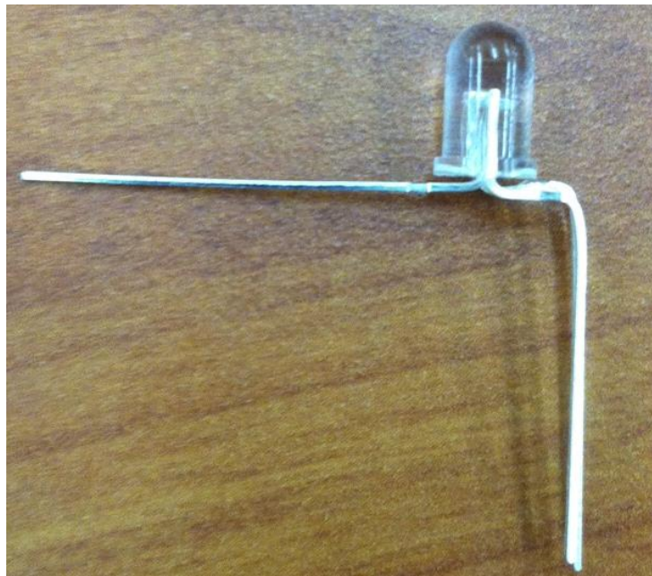
Figure 6.5: Illustration of LED lead bending.
