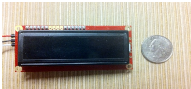
Fig. 3 Sparkfun Electronics 16X2 LCD Display used for guest and security tags
