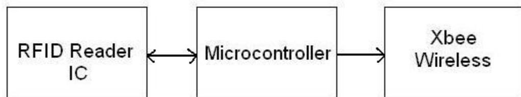
Figure 14 - Reader Unit block diagram
