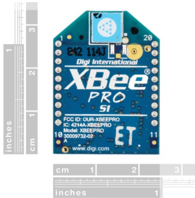
Figure 9 – Size comparison of the Xbee pro (Reprinted with permission from sparkfun.com)
