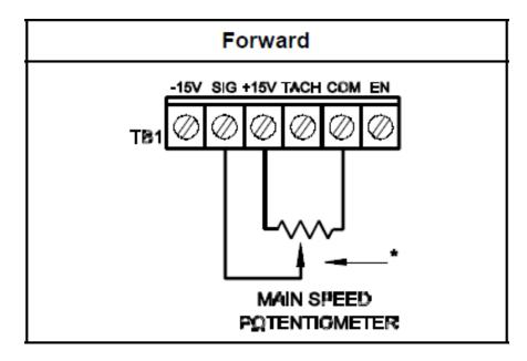
Figure 5.1.3.2a Speed Control Circuit
