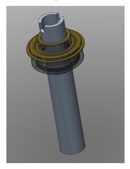
Figure 5.1.1.4a Bearing Assembly
