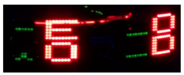
Figure 7.5.7c: RGB Text Array displaying alternating color text.
