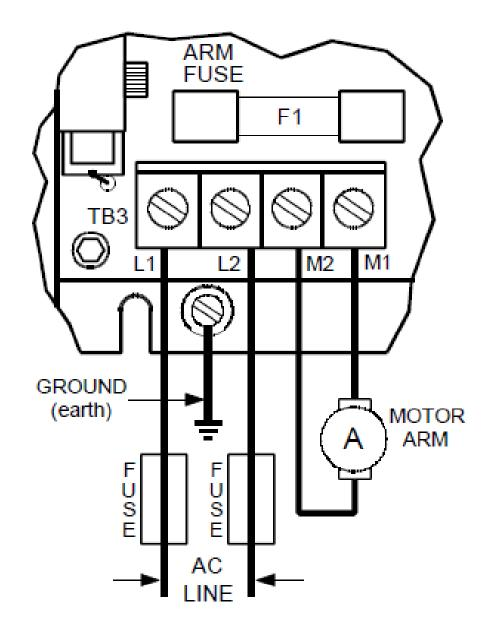
Figure 5.1.3.1a Motor and Power Connection
