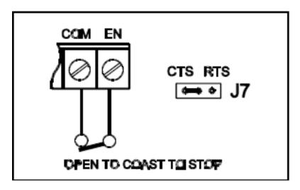
Figure 5.1.3.2b Enable Circuit
