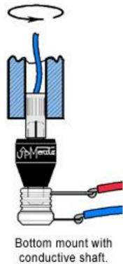
Figure 4.4.2.2.2 Model 205 Rotary Joint for Rotary Interfaces
