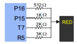
Figure 4.2.1.2.b Resistor circuit providing 16 colors from 4 inputs
