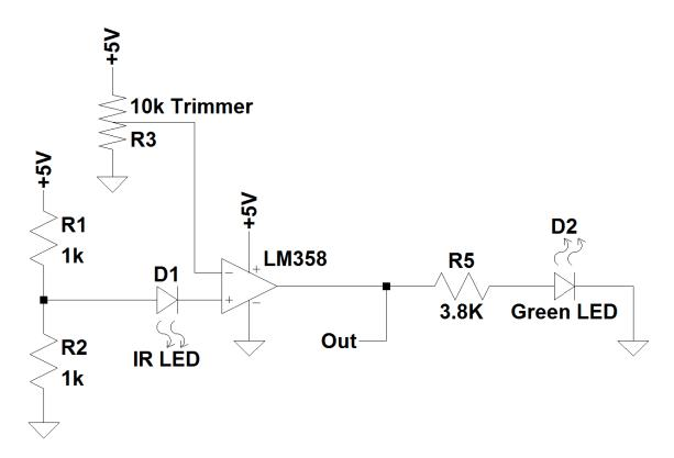
Figure 5.1.4c Display Alignment Receiving Circuit
