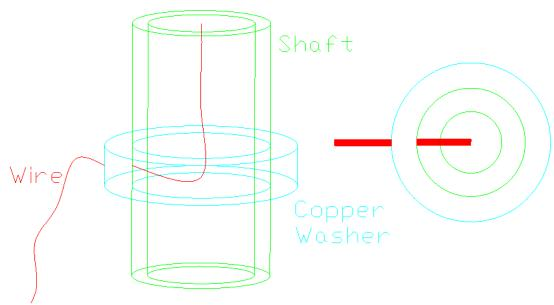
Figure 5.1.5.3a Slip Ring side and top view
