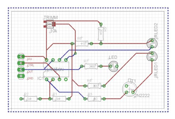
Figure 5.1.4d Display Alignment PCB Layout
