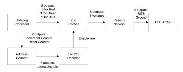
Figure 4.3.1.2 Latch control Implementation
