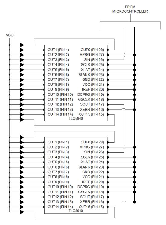
Figure 5.1.2.1b LED Controller Wiring
