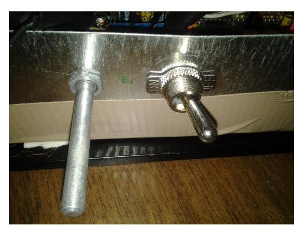
Figure 8.1 KBRG-212D Input Switches
