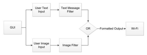
Figure 5.2.3 Pipe and Filter Software Architecture
