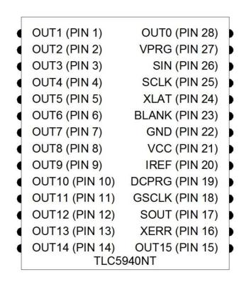
Figure 5.1.2.1a TLC5940 LED Controller Pin Out
