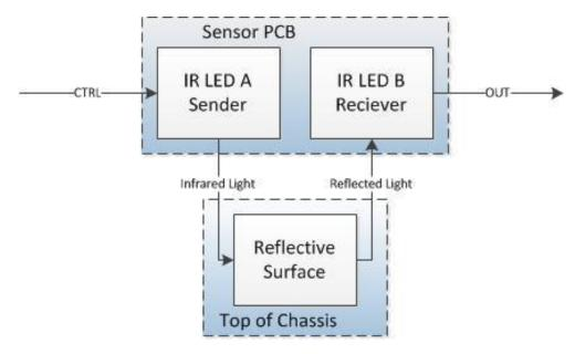
Figure 5.1.4a Display Alignment Sensor Flow Chart
