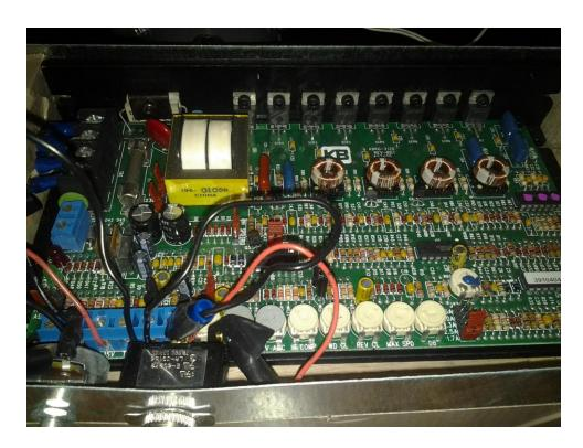
Figure 5.1.3b The KBRG-212D Regenerative Drive Chip
