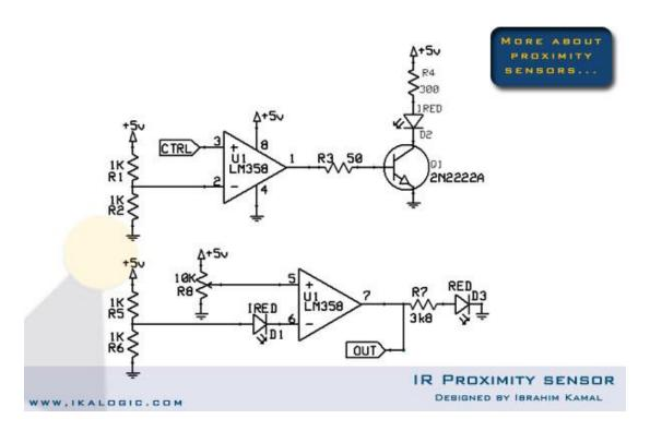
Figure 10.a Infrared Sensor Reference Circuit
