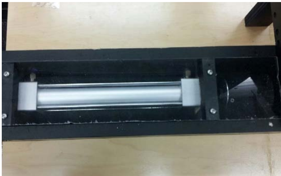
Figure 10: Can Crusher Pneumatic Cylinder
