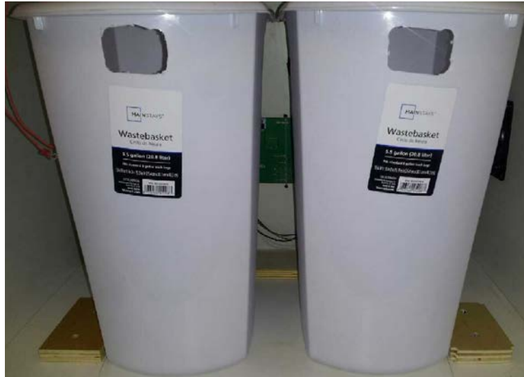
Figure: 33 Storage bins cut outs for storage sensors
