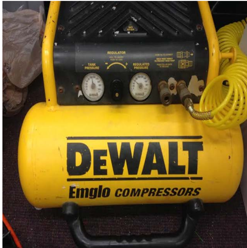
Figure 42: Air compressor for the project
