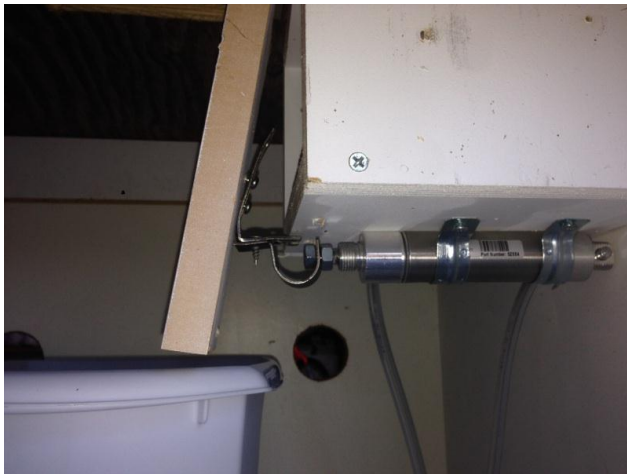
Figure 10. Shows the technique of the “swinging lid”. The pneumatic cylinder is connected to a movable plate that will direct which bin the object is stored in
