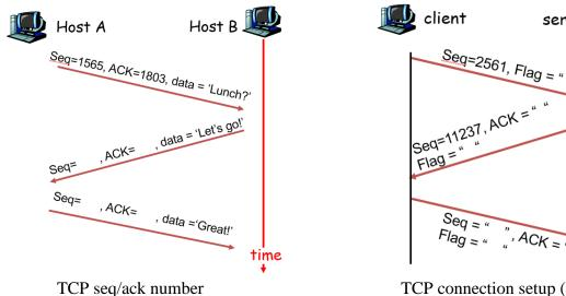
TCP connection setup (Flag are the values used in TCP packet header flag field)
