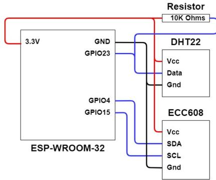
Fig. 5: Schematic of ESP32 with ECC608 and DHT22.
