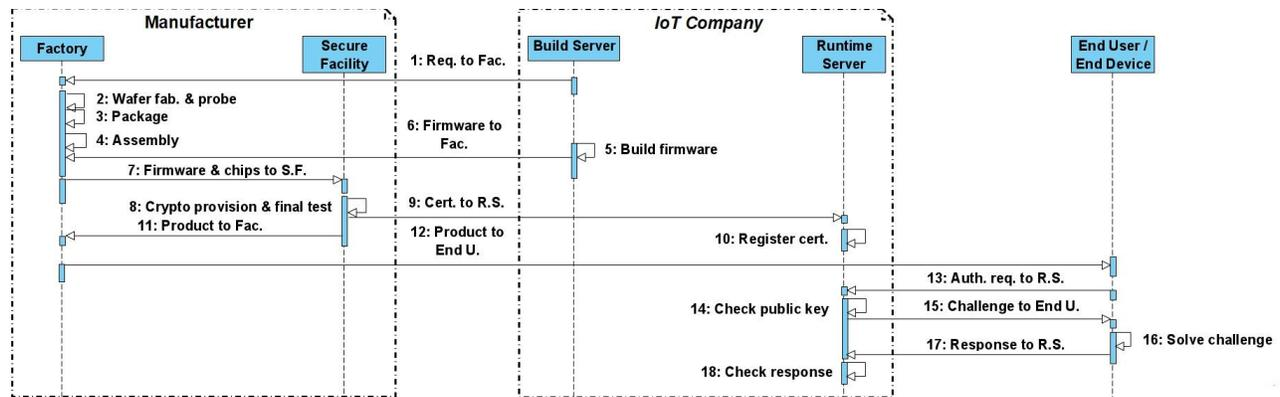
Fig. 4: Secure key provisioning framework.
