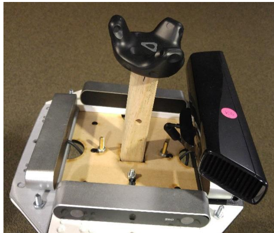
Figure 4. Mounting of sensor array with Kinect and Vive tracker for data recording sessions.
