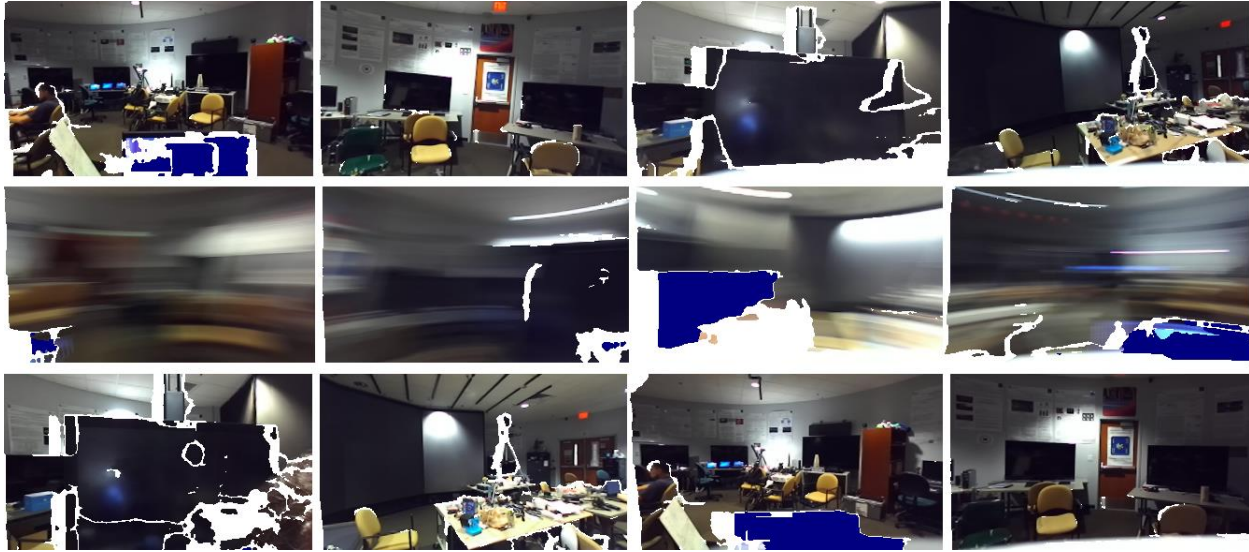
Figure 6. Example of extreme agile movements. The top frame is a normal color frame, the middle is during a 180-degree transition and the bottom set is once the transition has ended.
