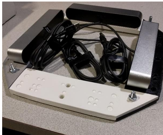
Figure 3. Arrangement of ZED sensors on 3-D printed platform. Fourth sensor is removed to show an example of the platforms.
