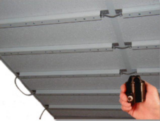
Fig. 1. The HiBall™ Tracking System. The tracker consists of a set of small, high speed cameras. The room is instrumented with a set of precisely surveyed rails. Each rail contains a set of infrared LEDs which are fired in a predetermined sequence.
