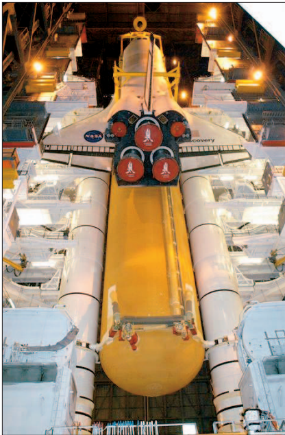
Figure 3. Inside the vehicle assembly building, NASA technicians lower the orbiter Discovery in front of the solid rocket booster and external tank already stacked on the top of the mobile launcher platform. After Discovery has been mated to the external tank and solid rocket booster assembly on the MLP and all umbilicals have been connected, workers will electrically and mechanically verify the mated interfaces to ensure all critical vehicle connections.
