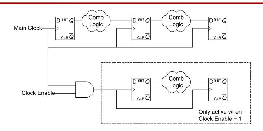
Clock gating is a direct means for reducing dynamic power dissipation but
