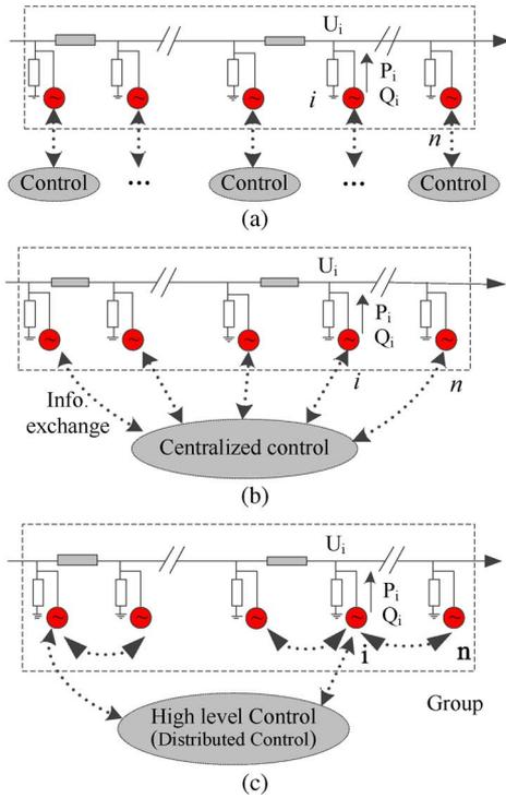
Fig. 1. Three different control modes in a distribution network (the dash arrows represent information flow). (a) Decentralized mode. (b) Centralized mode. (c) Distributed control mode.
