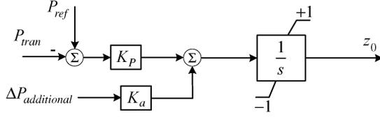
Fig. 5. Control determining the desired ratio of P.
