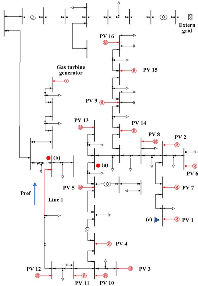
Fig. 6. Diagram of the IEEE 34-bus network.
