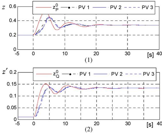
Fig. 12. Responses to intermittent communication and load changes. (1) Active power ratios of PVs 1–3. (2) Reactive power ratios of PVs 1–3.
