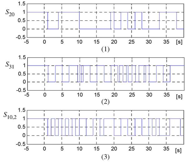
Fig. 10. Intermittent interruptions in communication channels.
