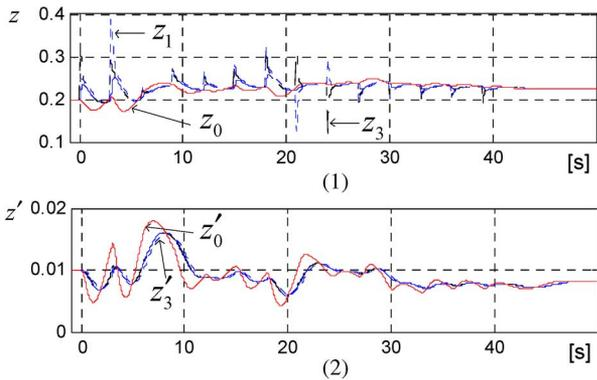
Fig. 9. Responses to sunlight changes: (1) Active power ratios of PV 1, PV 3, and  $\alpha_P^0$ . (2) Reactive power ratios of PV 1, PV 3, and  $\alpha_Q^0$ .
