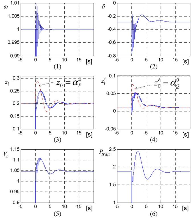
Fig. 7. Dynamic responses under fault (a): (1) Frequency of gas-turbine generator. (2) Angle of the gas-turbine generator. (3) Active power output ratios for PV generators 1 to 4. (4) Active power output ratios for PV generators 1 to 4. (5) Critical bus voltage. (6) Active power transmitted over line 1.
