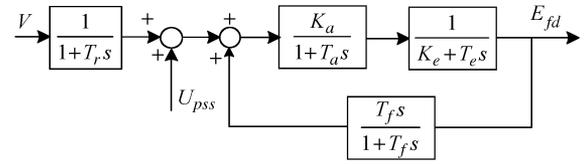
Fig. 13. Transfer function of IEEE-1 exciter.
