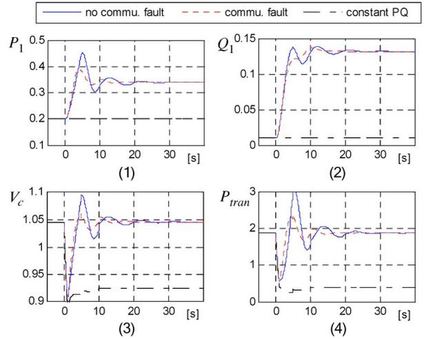
Fig. 11. Responses to load changes with and without intermittent communication.
