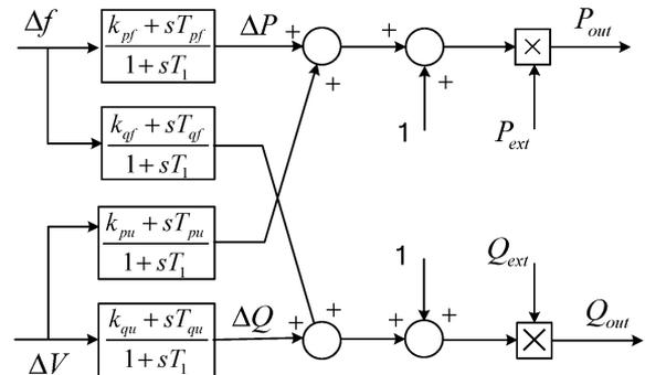
Fig. 16. Transfer function of load dynamics.
