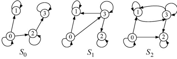
Fig. 3. Graphs for time-varying communication topologies.
