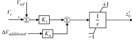
Fig. 4. Control for determining the desired ratio of Q.
