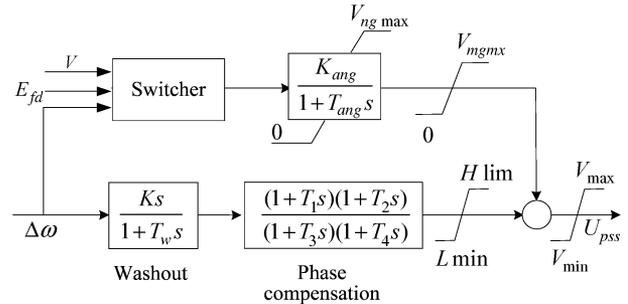
Fig. 14. Transfer function of PSS-ostab2.
