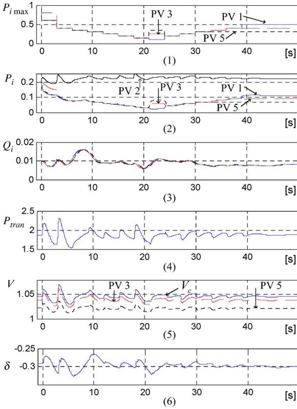
Fig. 8. Responses under sunlight changes: (1) Sunlight changes. (2) Active power outputs of PV generators 1, 2, 3 and 5. (3) Reactive power output ratios of PV generators 1, 3, and 5. (4) Active power across line 1. (5) Voltages at the critical buses. (6) Rotor angle of the gas-turbine.
