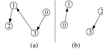
Fig. 2. Sample graphs of communication topology. (a) Existence of one globally reachable node. (b) Absence of globally reachable node.
