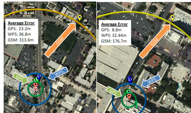
Figure 1: Accuracy of GPS, WPS, and GSM-based Positioning
