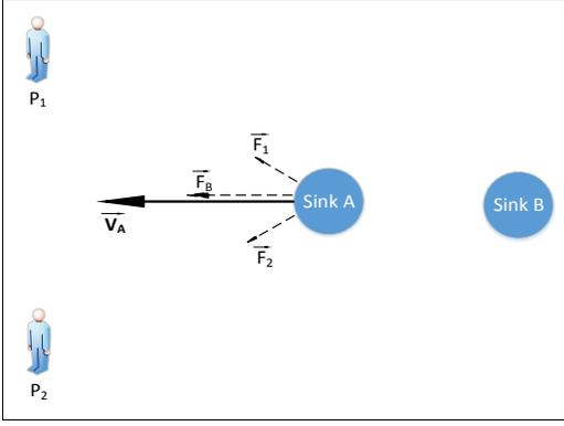
Fig. 4. The physical forces and movement vector of *Sink A* along with pedestrians  $P_1$ ,  $P_2$  and *Sink B*.
