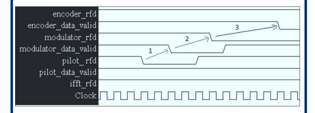
Stall caused by piloting block propagating backwards
