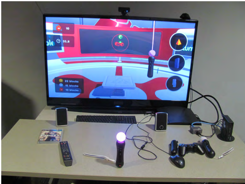
Figure 3.1: The experimental setup used a Samsung 50 inch DLP 3D HDTV, PlayStation 3 game console, PlayStation Move controller, and a Mitsubishi 3D adapter (to convert the HDMI 1.4a 3D signal to a DLP 3D signal). These are all commodity hardware components.
