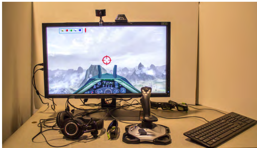
Figure 6.4: The experiment setup consisted of a 27" BenQ XL2720Z 3D monitor, Nvidia 3D Vision kit, a TrackIR 5 with Pro Clip (mounted on a headphone), a Logitech Extreme 3D Pro joystick, and a PC (Core i7 4770K CPU, GTX 780 graphics card, 8 GB RAM).
