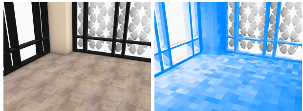
Figure 6: (Left) An example BIM data visualization of our test building environment with a facade design in place. (Right) An example daylighting radiation analysis applied. The BIM data is matched in reality to visualize the designs and daylighting in AR.
