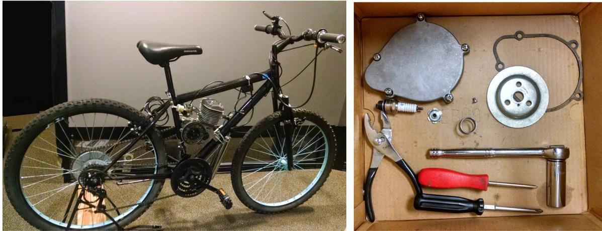
Figure 5.2: The physical motorized bicycle apparatus (5.2a) with the accompanying tools and parts (5.2b).
