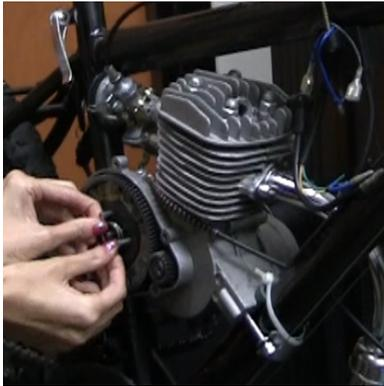
Pressing and rotating the spring over the center bolt until it clicks into place
