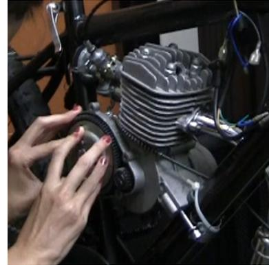
Tightening the clutch wheel nut over the clutch plate to the appropriate tightness
