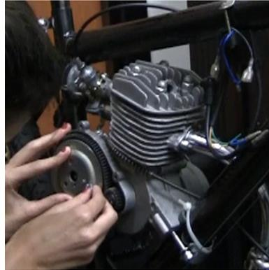
Pressing and aligning the clutch plate over the spring and three pegs
