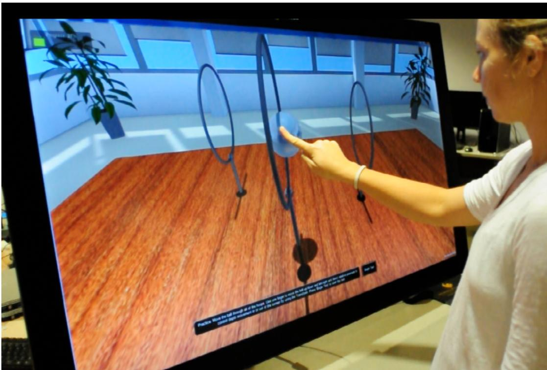
Figure 4.1: Our experiment apparatus included a 55-inch Perceptive Pixel display raised to standing height and tilted upwards by 30 degrees.
