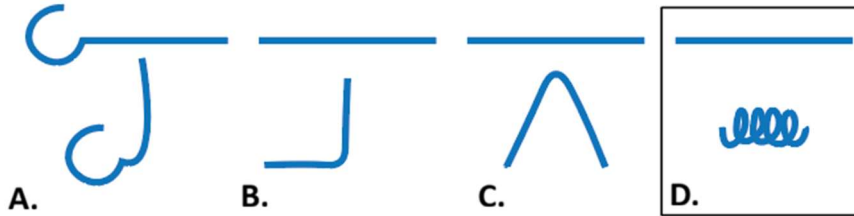
Figure 3 – All attempted Nitinol shapes (at rest above, actuated below). Bending straight upwards with an eyelet for sewing (A), bending at a 90 degree angle with flat ends (B), bending into a downward arch (C), and coiling into a spring (D).
