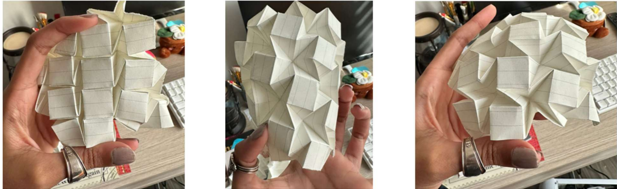
Figure 2 - Waterbomb tessellation folded from paper. At rest (left), pulled into a cylinder (middle), and pulled into a hemisphere (right).
