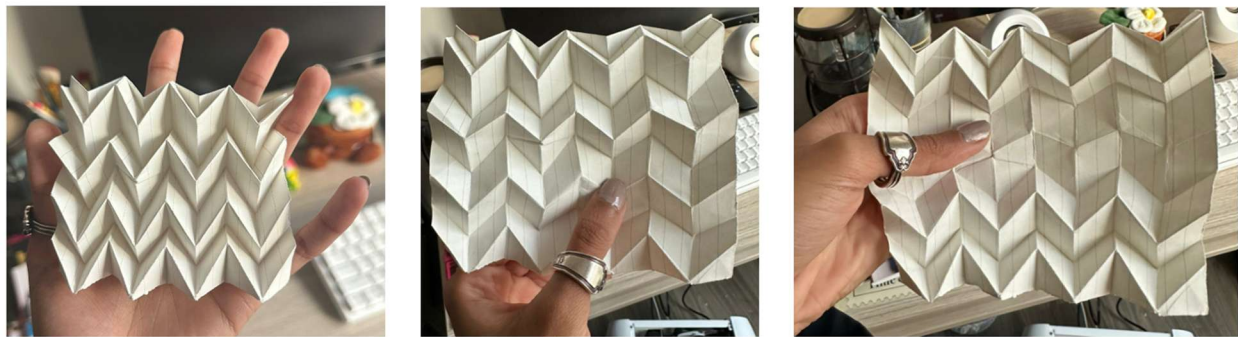
Figure 1 - Miura Ori tessellation folded from paper. At rest (left), with one cell flattened (middle), and with one row flattened (right).
