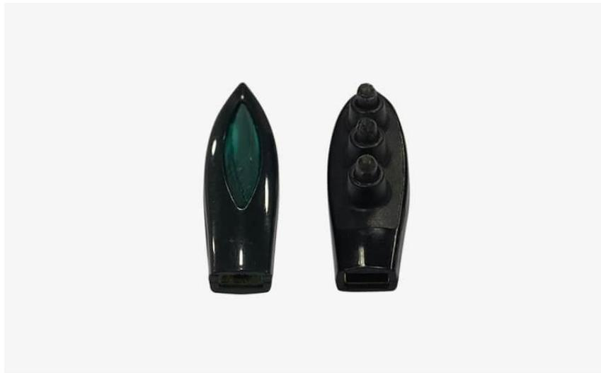
*Figure 3: Emotiv Insight II polymer sensors: three-pronged (left), one-pronged (right).*
