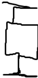
Figure 22 – Example of duplicated points and self-intersections
