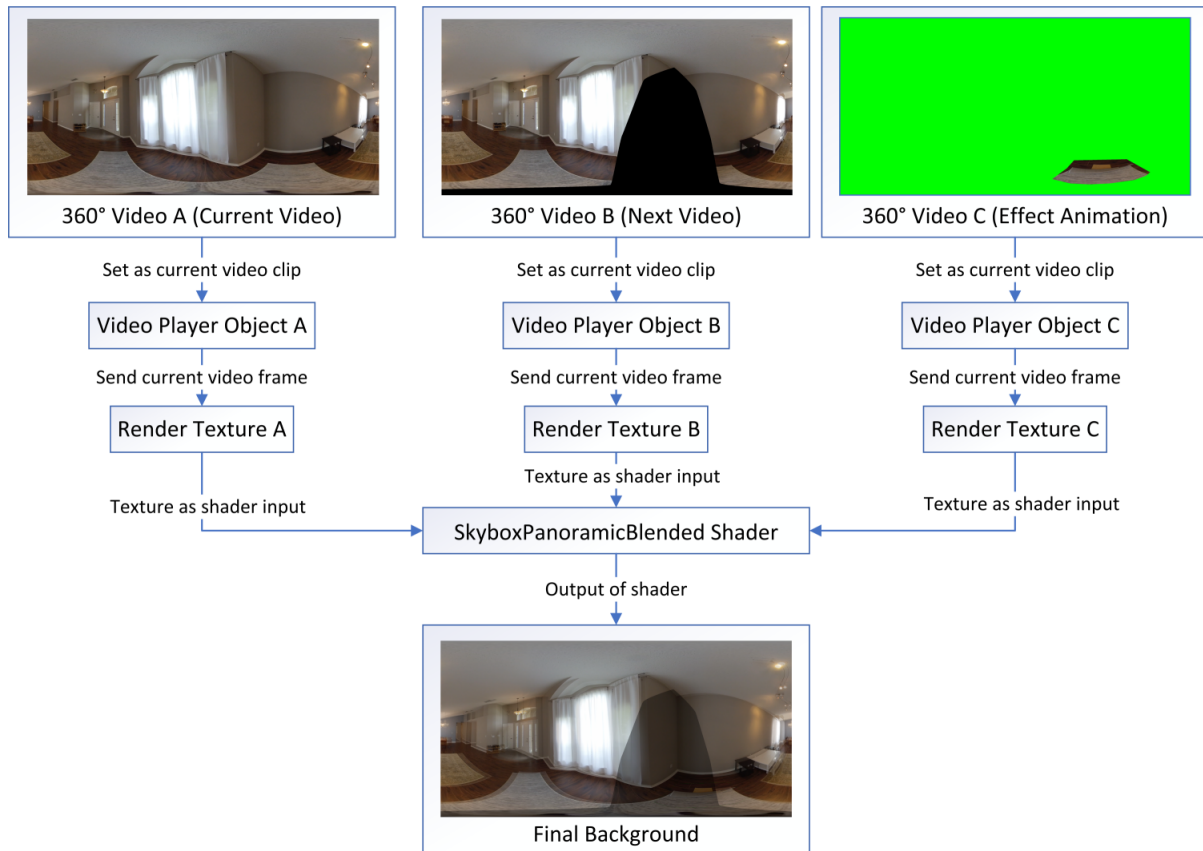
Figure 3.6: The Video Manager render pipeline, illustrating the high-level process of how the 360 VR environment is made.
