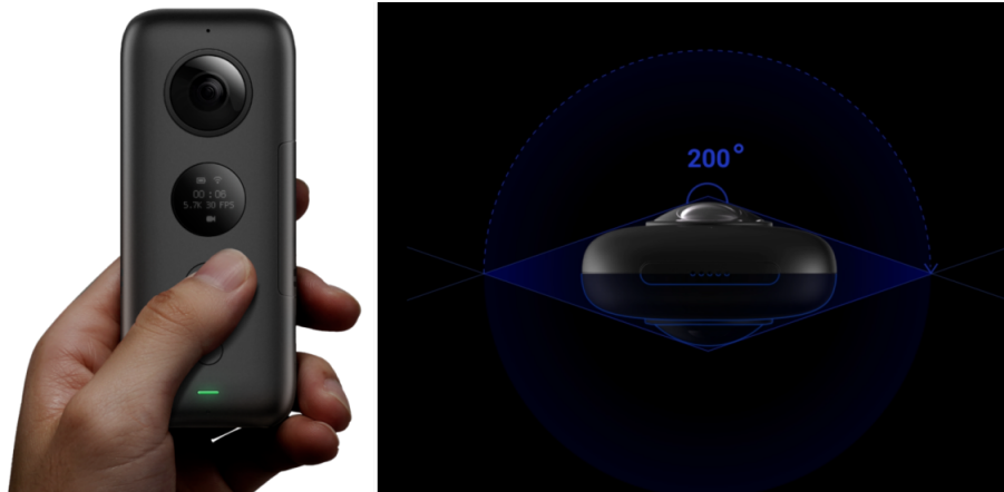
Figure 3.1: Side and top view of Insta360 One X. Illustrates the viewing angle for each lens.
