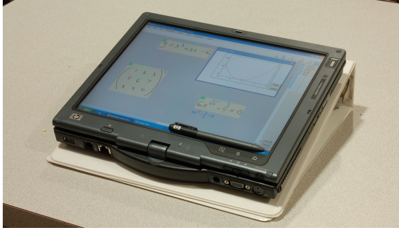
Figure 2: A Compaq tc4400 Tablet PC, running AlgoSketch, set at a 15 degree angle on a 2 inch high binder.
