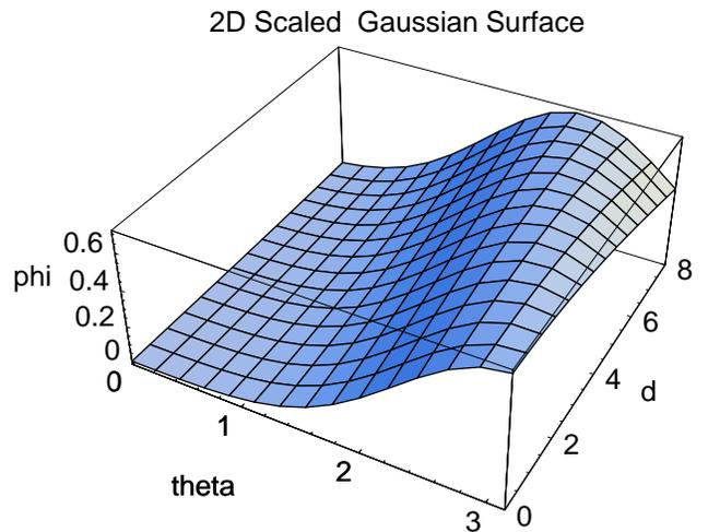
**Figure 7** A visual representation of the scaled 2D Gaussian surface we use to find the rotation factor, which determines the degree of rotation amplification. For this graph,  $\sigma_1$  equals 0.57,  $\sigma_2$  equals 0.85, and  $L$  equals 30.
