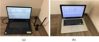
Fig. 2. Two ways of setting up out-of-network capturing. (a) Sniffing using Alfa WiFi interface and either Airodump-ng or Kismet software.(b) Sniffing using MacBook built-in WiFi interface and Airtool software.
