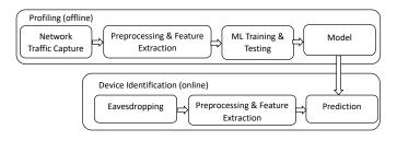
Fig. 1. IoT device profiling attack system.
