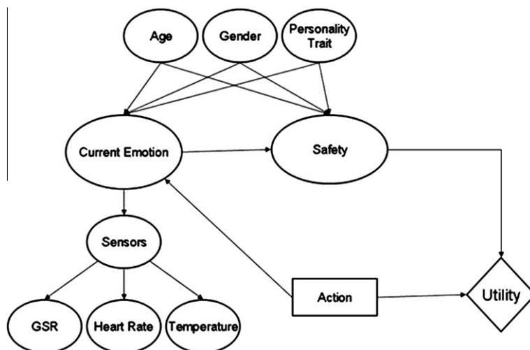
Fig. 17. Bayesian Belief Network representation for user model of a driver.
