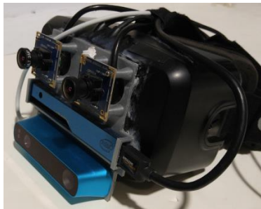
Figure 4. Oculus Rift HMD modified with sensors used in the experiment.
