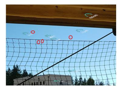
**Figure 6.** An example of enhanced situational awareness via augmented reality. Red circles were added in to illustrate the physical location of unmanned aerial vehicles that were reporting their GPS coordinates to the network. Photo was taken at FX4 event in Washington as live footage from FX6 event in Fort Campbell, Kentucky was not available.
