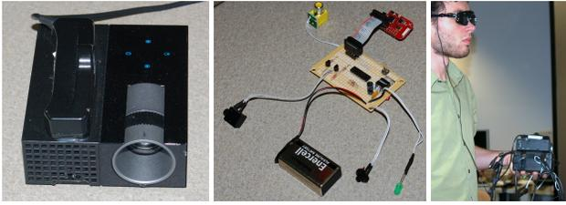
Figure 2: Hardware components: (left) handheld projector with attached tracking device; (center) custom microcontroller board for synchronizing shutter glasses; (right) user holding the microcontroller board and projector, wearing shutter glasses
