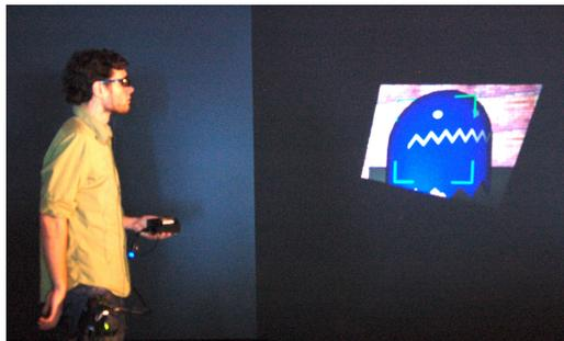
Figure 1: A user of our prototype system for interacting with objects in a 3D virtual world. The virtual world is revealed wherever the user points the projector. The 3D ghost is revealed when the users points the handheld projector in a given location on the screen. Although the projector is clearly oblique to the projection surface, the crosshairs appear orthogonal because of compensation using the tracker.
