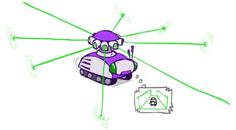
Sensor model: can read in which directions there is a wall,
