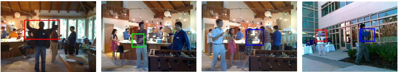
Figure 6: Examples of action detections on MSR dataset using VP+TPSS. Colored boxes denote detected actions: boxing (blue), clapping (green), and waving (red). Qualitatively, our results are comparable to Cao et al. [3].
