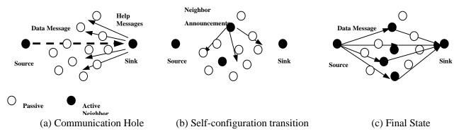
Figure 1. Simplified schematic of a self-configurable sensor network.
