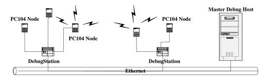
Figure 3. Basic Testbed configuration
