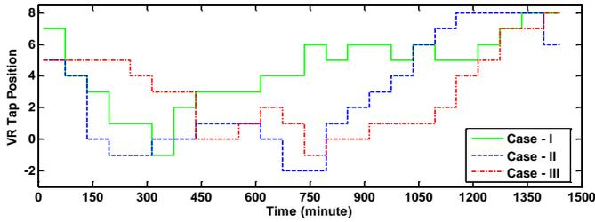
Figure 6. Voltage regulator tap position in three cases.
