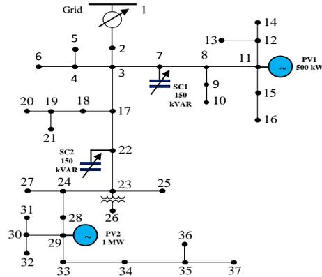
Figure 3. One line diagram of test system.
