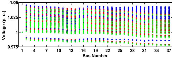
Figure 7. Voltage profile in case I (red, blue, green: phase a, b, c).
